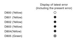
• : ON, O : OFF, (a) :Rapid flashing (5 times / second)
